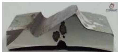
A typical MIC failure observed in a SS316L pipe in water service
